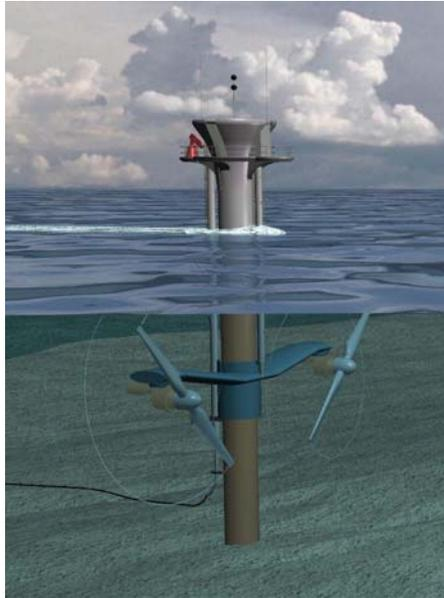
Fig B: Artists Impression of a MCT Seagen pile-mounted twin rotor tidal turbine
