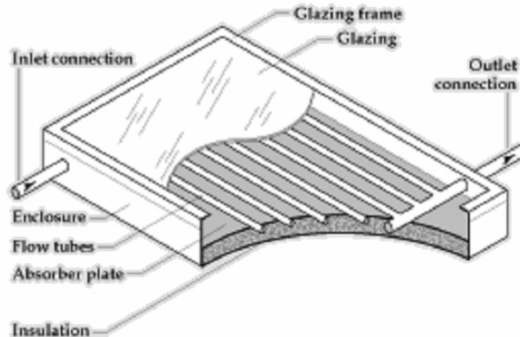
Fig H: Flat Plate Collector
