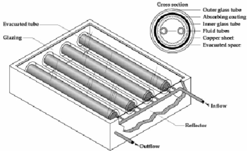
Fig 1: Solar Evacuated Tube Collector
