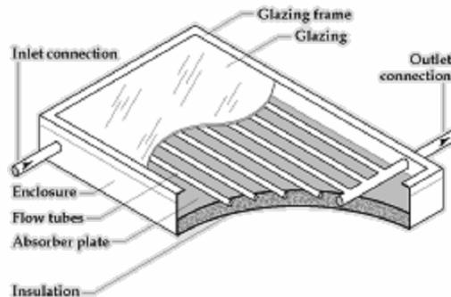
Fig 9: Flat Plate Collector
